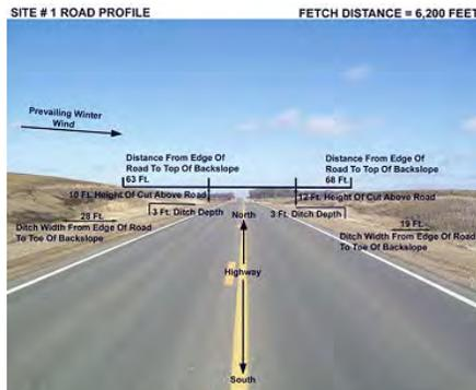
An online tool is available to help transportation agencies design drift-free roads. The Minnesota Drift-Free Roads Design Module allows user to create two types of mitigation strategies: a proper road design and a snow fence design.
