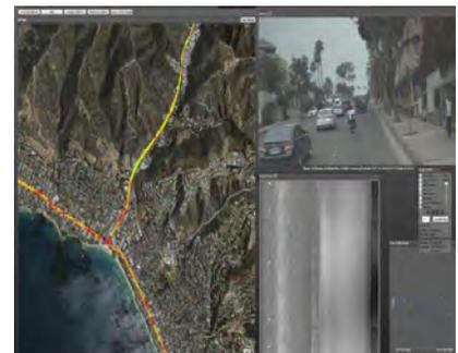
Figure 2. Image of the Automated Pavement Condition Survey Showing IRI Color Ratings of the Highway, and also Forward and Downward Photo Images
