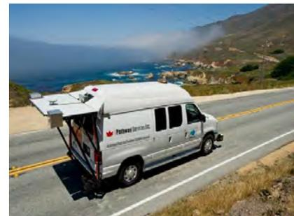
Figure 1. Caltrans Instrumented Van for Pavement Condition Rating
